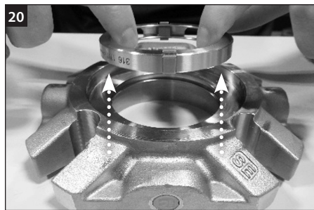
从压盖上取下传动沟槽；从传动沟槽上取下沟槽夹和导流板并丢弃。
